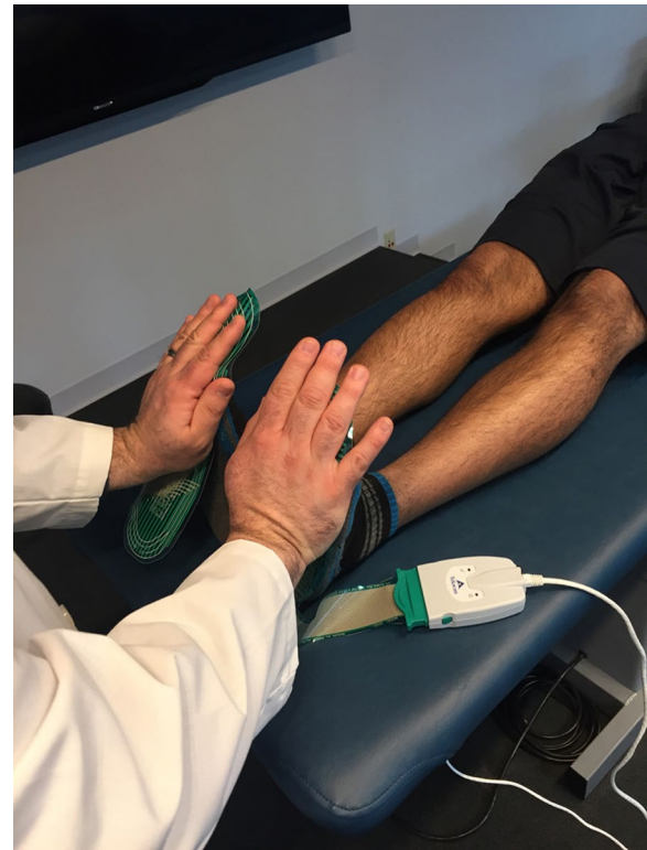
Fig. 2 F-scan system to measure force
